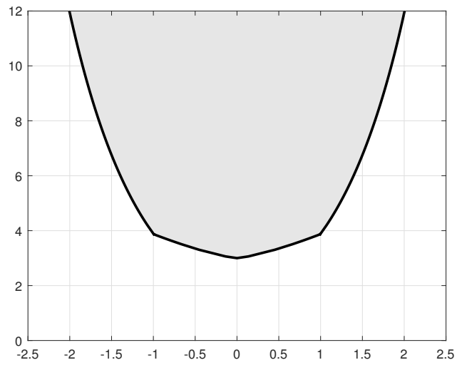
Figure 14: The joint range skewness-kurtosis. Levels for skewness are on the x-axis, whereas those for kurtosis on the y-axis.
